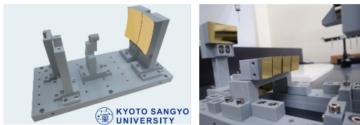
Combination of Mirrors and Structural Components by Cordierite
