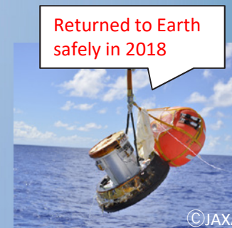
Thermal Protection System for HTV Small Re-entry Capsule
