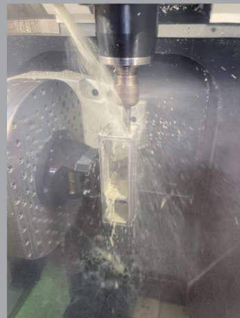
ex. 3U CubeSat Structure during Processing
